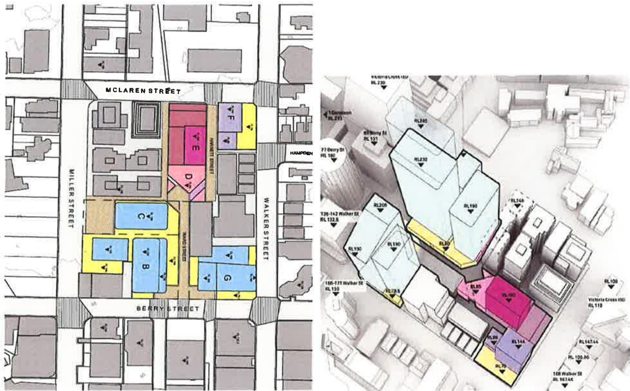
Figures 6 and 7: Miller Street Square masterplan option (brown areas are public domain) (left) and proposed built form envelopes as viewed from the east (right).
